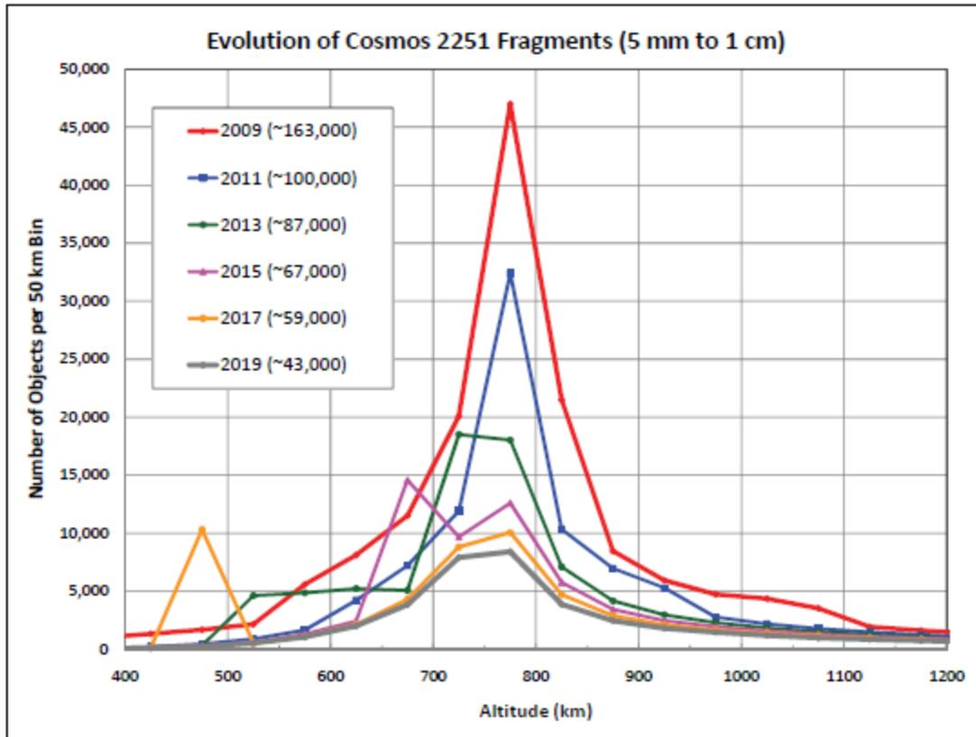
Figure 1. Altitude distributions of the simulated 5-mm-to-1-cm Cosmos 2251 fragments between 2009 and 2019. The number of remaining in-orbit objects at each snapshot is indicated in parenthesis.
