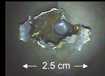
Shuttle radiator damage, 2007
